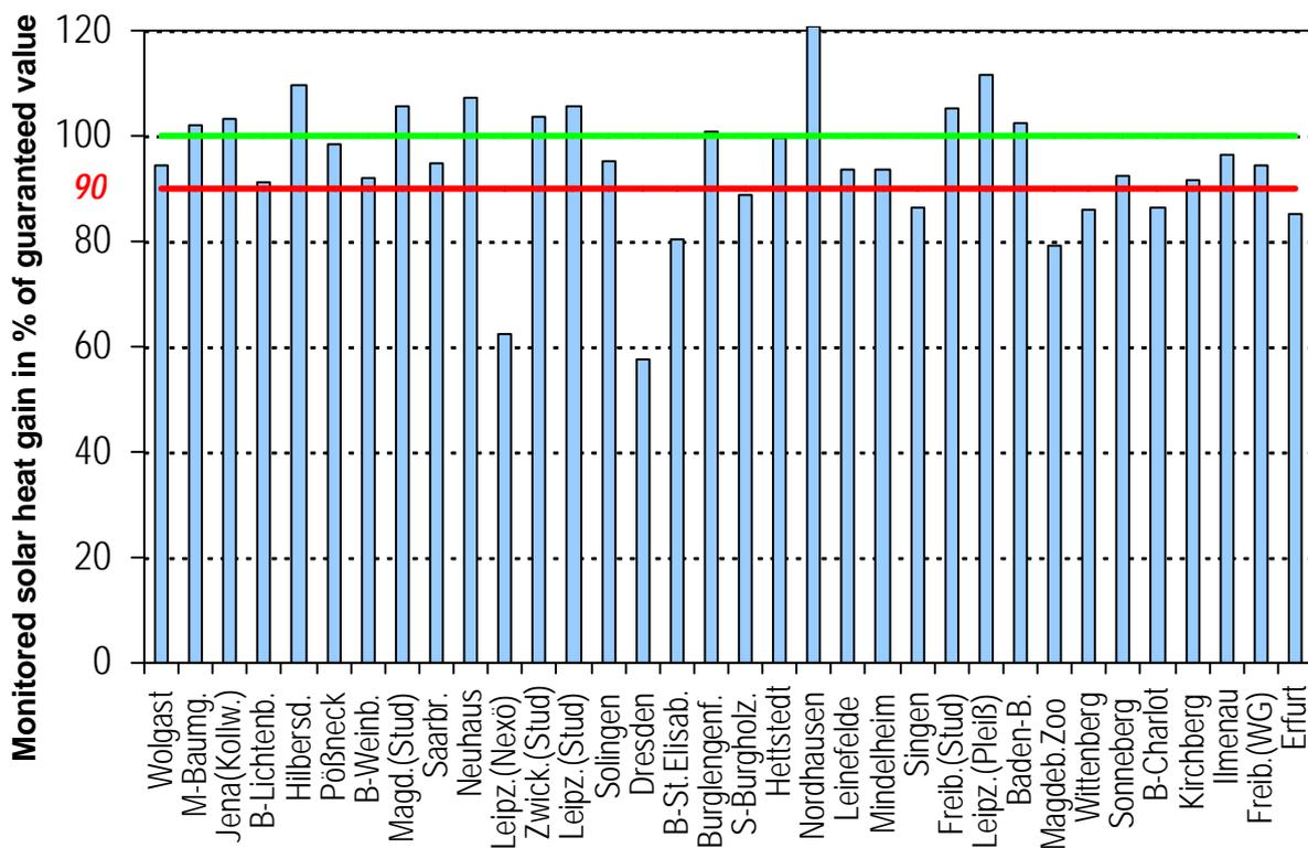
Figure 2: Monitored solar heat gain in % of the recalculated guaranteed value for the pilot plants of Solarthermie-2000 part 2.
