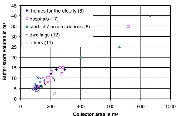
**Figure 1: Plants of Solarthermie-2000 part 2 in operation (in brackets the amount of plants)**
